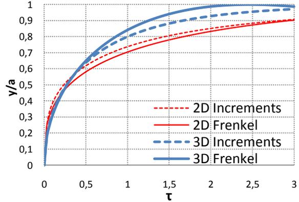
**Fig. 2.** Comparison between 2D and 3D Frenkel model.
