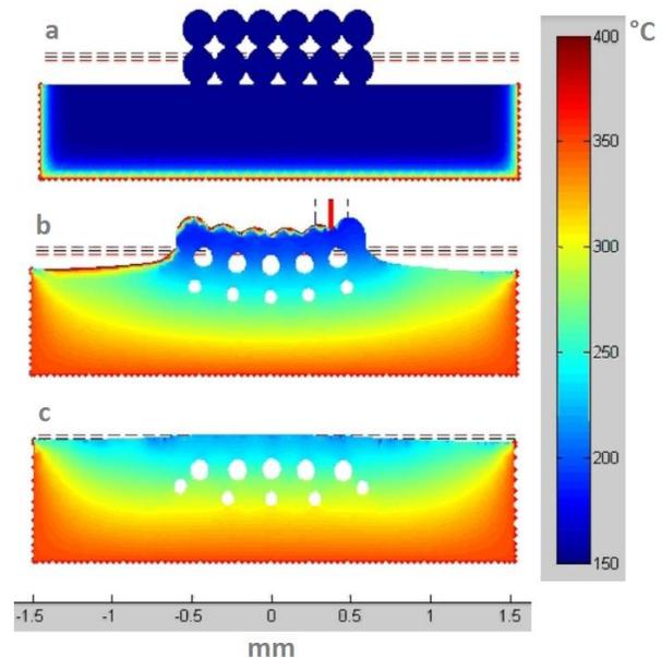
**Fig. 6.** Captures of simulation evolution (a - solid polymer, b - laser pass, c - melted polymer) during the SLS process applied on 12 cylinders.
