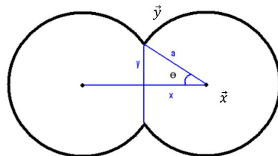
**Fig. 1.** Shape of two cylinders during coalescence - Definition of parameters.
