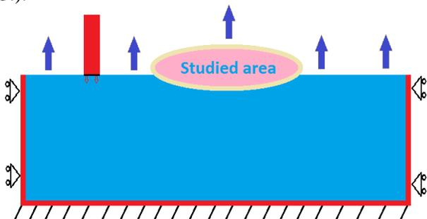
**Fig. 3.** Thermal and displacement limit conditions of the simulation
